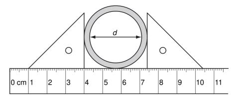
What is the internal diameter *d* of the tube?
