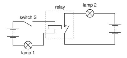
When switch S is closed, what is the state of the lamps?
